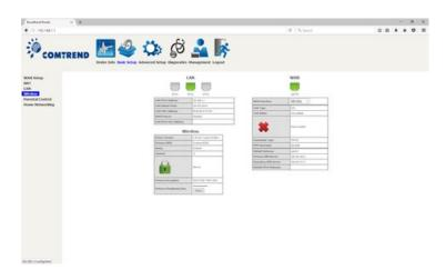
3) Check mark "Enable Wireless", and change the "SSID" if you wish, then click "Apply/Save". (By default, wireless is disabled but the SSID is ComtrendXXXX, where XXXX are replaced with the last 4 characters of your routers MAC address).
